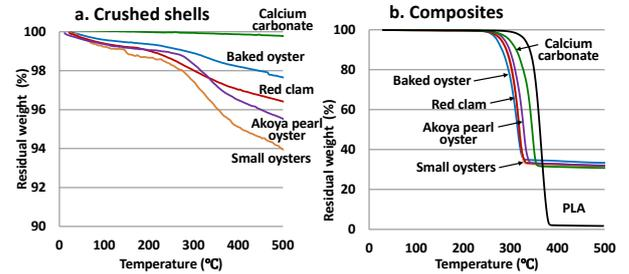
Fig. 4 Thermogravimetric analysis of crushed shells and composites
