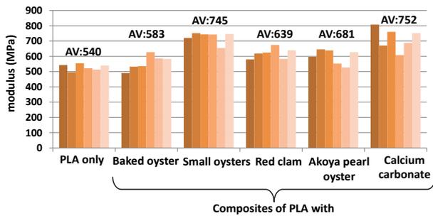
Fig. 2 Tensile test results (modulus of elasticity)
